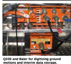
Q330 and Baler for digitizing ground motions and interim data storage.
