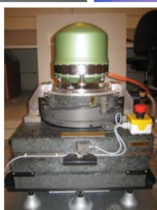
The 3-component calibration table determines the seismometer constant. Developed by Edi Mayer & Partners/Switzerland and Föhrenbach/Germany in collaboration with Prof. Erhard Wielandt and DI Gunnar Streckelsen.
